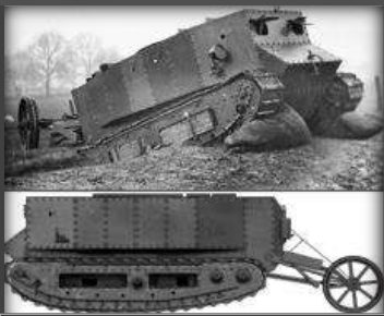
World's first tank, Little Willie. It lacked a turret on top and the top speed was 3,2 km/h. These vehicles were called landships at the time.
